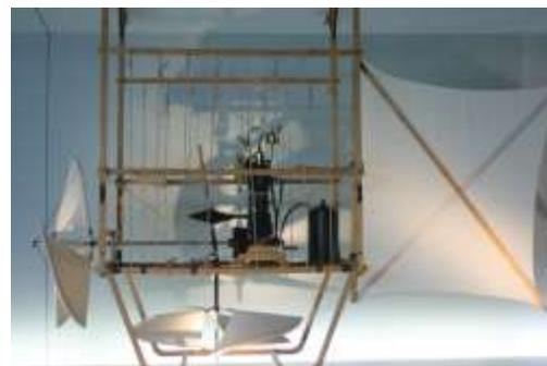
Daimler’s “Grandfather Clock” Engine Powered the First Boat and Airship
